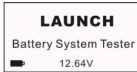
Figure 1 Startup Interface with Voltmeter On
