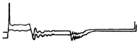
Secondary circuit cut-off intermittently
