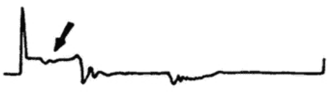
Mixture ration is too lean or cylinder pressure is too low
