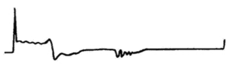
Ignition coil or capacitor leak voltage
