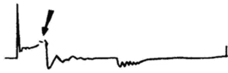
Spark plug overheated or valve guide leakage
