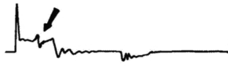
Distributor cover or distributor lead is matched un-tightly
